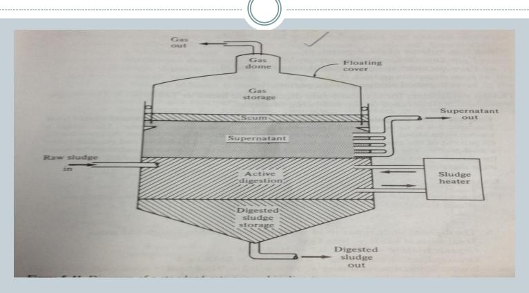
• Sludge is fed into the digestor on an intermittent basis and supernatant is withdrawn and returned to secondary treatment unit
